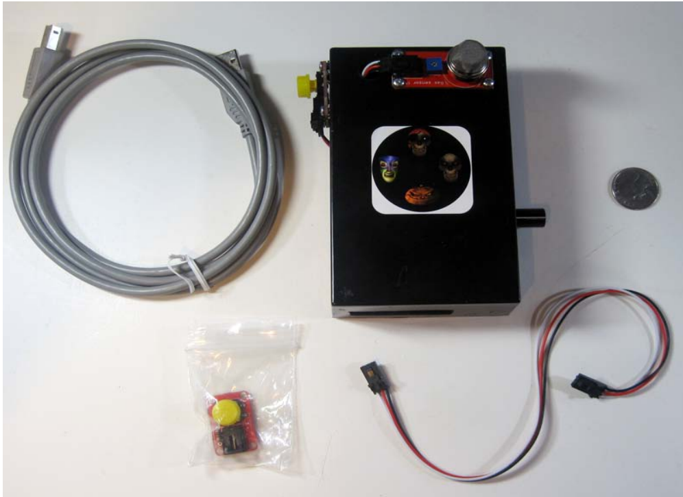
Figure 1 – Assembled Magic Mirror Sensor Hub with Case (Yellow Push Button and Cable Not Included)
